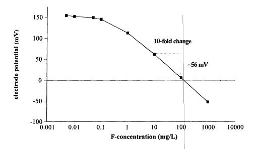
Fig. 3.1 Typical standard curve obtained with the F ion-specific electrode (Orion, model 96-09)
