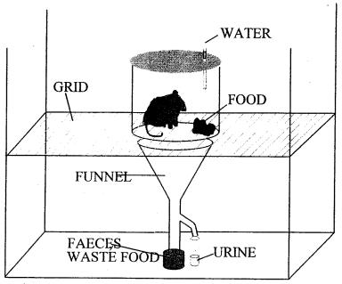
Fig. 3.3 Diagram of metabole used to collect gerbil urine
